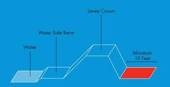
Anatomy of a levee: Levee cross-section depicting the minimum 10 foot maintenance and flood fighting easement.
