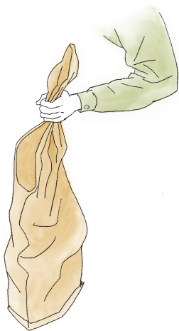
Figure 12A: Sandbag filled 1/4 to 1/3 full
